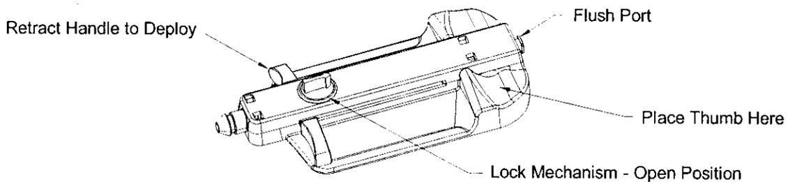
**Figure 3. Delivery System Schematic**
