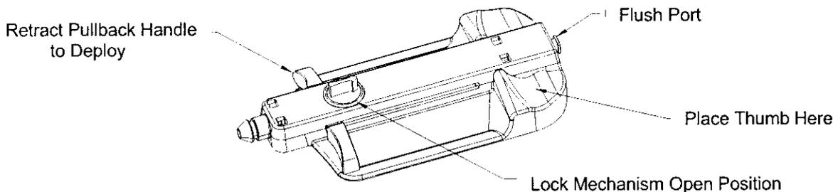
**Figure 3. Delivery System Schematic**
