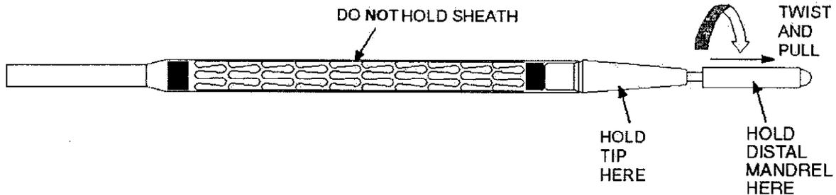
(Hold the tip to remove the distal mandrel.)
