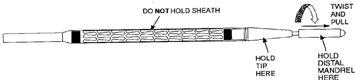
(Hold the tip to remove the distal mandrel.)
