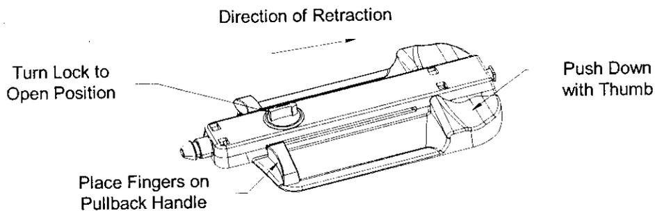
*With the guide position fixed, deploy with one hand.
